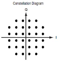
Fig 6. 32-QAM mapping
