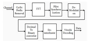
Fig.2 The OFDM receiver system
