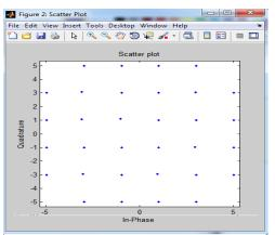
Fig 10. 32-QAM mapping
