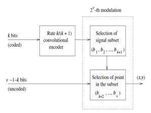
Fig 4 General encoder of rate(v-1)/v trellis code
